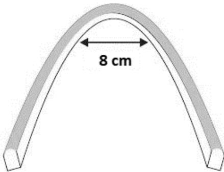
Figure 2 - The minimum bending diameter is 8 cm
