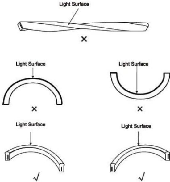
Figure 1 – Bending the LED neon flex 230V correctly
